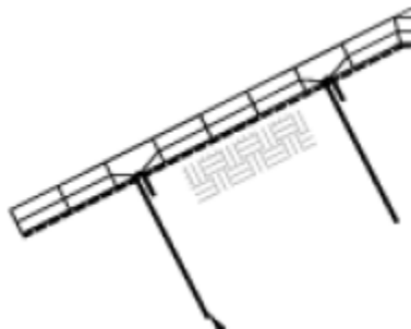
J HOOK ENGAGED TO TENDON FOR TENSION
