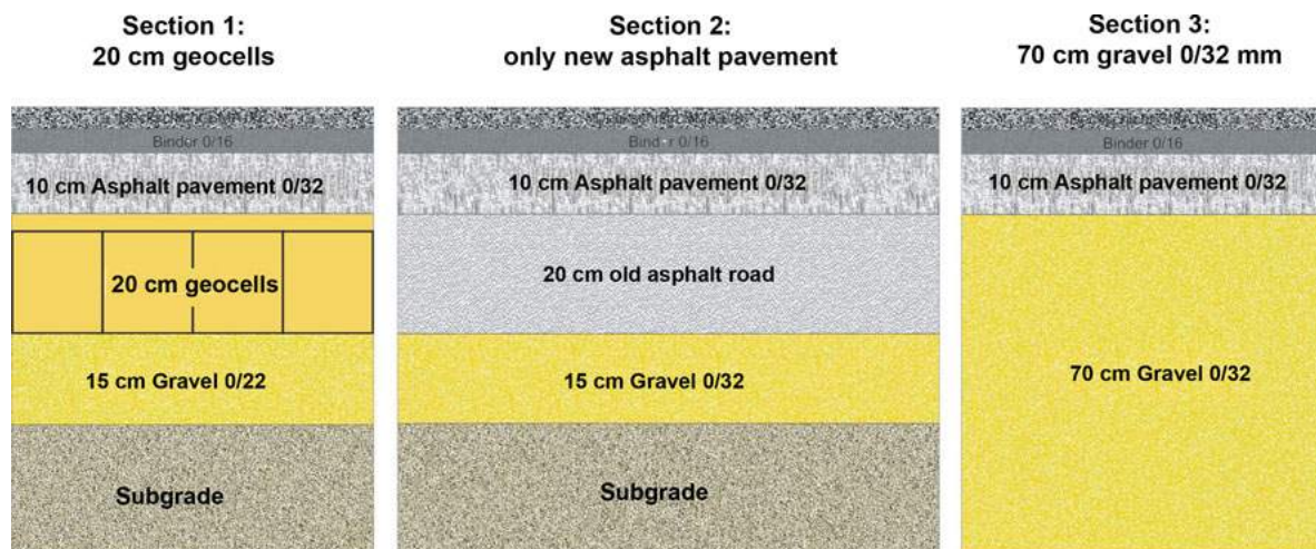
Figure 4: Different reconstruction section, road K-23.
